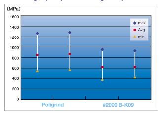
Workpiece: 8" silicon mirror wafer Z2 removal amount: 35 um Final thickness: 200 µm
