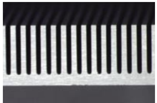
High-load deep-groove processing, which could only be realized with multi-step cutting, can now be processed in one pass.
