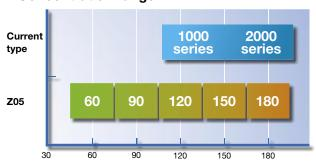
During dicing, grit concentration affects both the speed of blade wear and the size of chipping. By selecting precisely a grit concentration that is appropriate to the application, both wear speed and process quality can be made more stable and consistent. "Grit concentration" refers to the percentage of diamond grit in the abrasive portion of the blade. For example, a grit concentration level of 100 indicates 25% diamond grit by volume.
